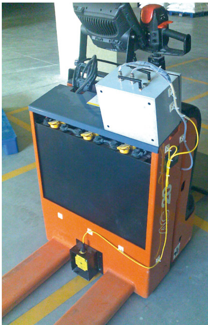
The read/write head at the forklift collects the data of the pallet and forwards it wireless over the BL67 I/O system to the PLC
