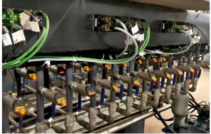
The sensor housing can be freely rotated by 340°, allowing convenient alignment of the display and electrical connection
