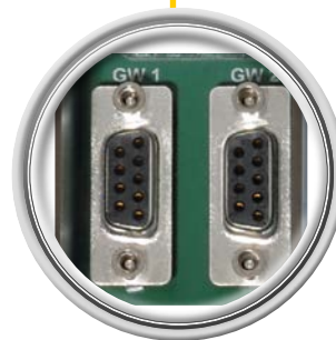
Connection of the higher-level PROFIBUS-DP fieldbus
