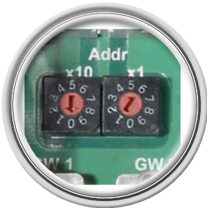
Choice of bus address via rotary coding switches or per software
