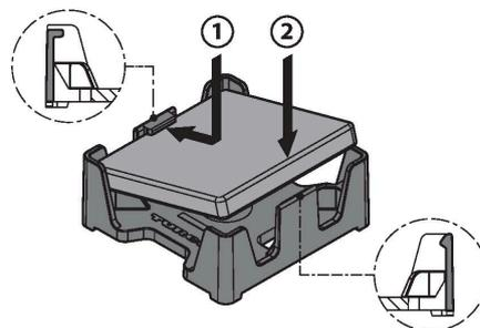
Mounting the data carrier properly in the retainer
