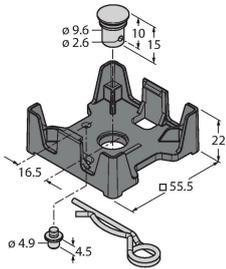
Retainer with spring cotter for Q51 tag. The use of the 4.5 mm lock pin ensures protection against twisting of the retainer or the tag For mounting on metal. Suitable for repeated use in high-temperature. Only suitable for a single assembly (engage the tag in the retainer). The use of the retainer results in a clearance of 12 mm between metal to tag.
