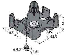
Retainer with M5 threaded bush to screw on Q51 tags. The use of the 4.5 mm lock pin ensures protection against twisting of the retainer or the tag For mounting on metal. Suitable for repeated use in high-temperature. Only suitable for a single assembly (engage the tag in the retainer). The use of the retainer results in a clearance of 12 mm between metal to tag.
