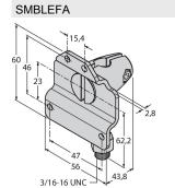
Mounting bracket, rotatable, stainless steel, for sensors of the LE250/550 series
