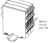
IMX12-AIO..-..-..0/... mount directly on the DIN rail.
