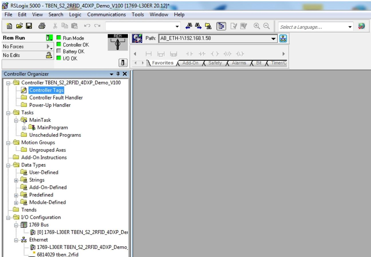
Fig. 30: Controller tags in the project tree
