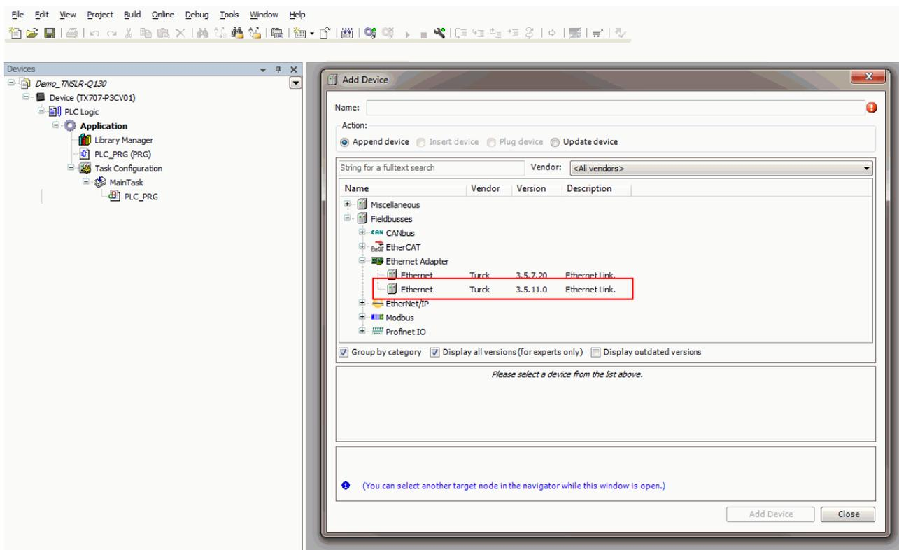
Fig. 15: Adding an Ethernet adapter
