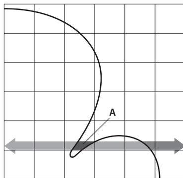
Fig. 38: Detection range of a read/write head
