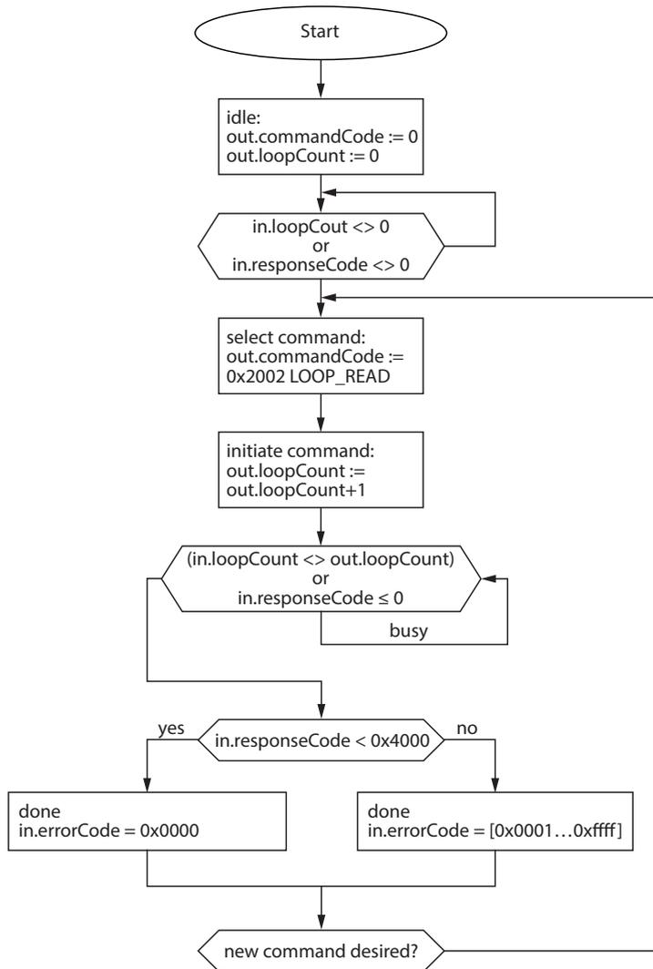
Fig. 56: Flow chart for fast command processing with loop counter
