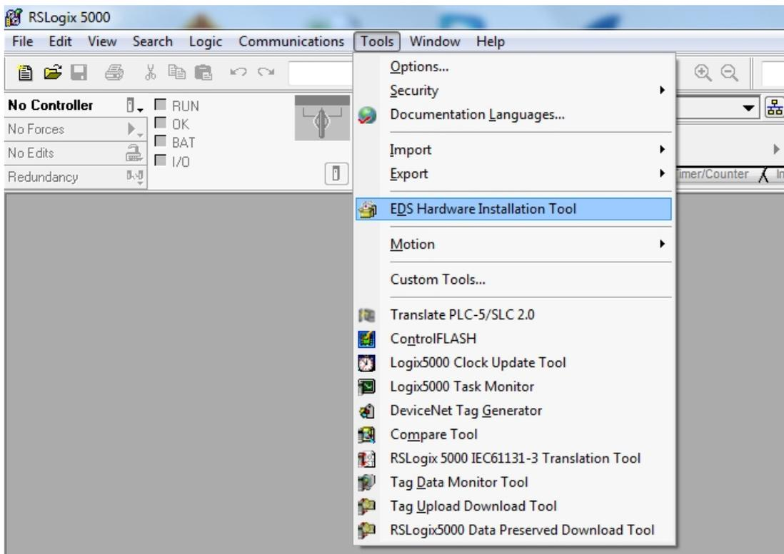
Fig. 26: Opening the EDS Hardware Installation Tool
