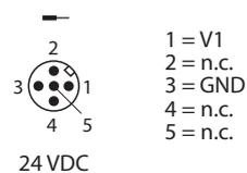
Fig. 9: Pin assignment for the power supply connection
