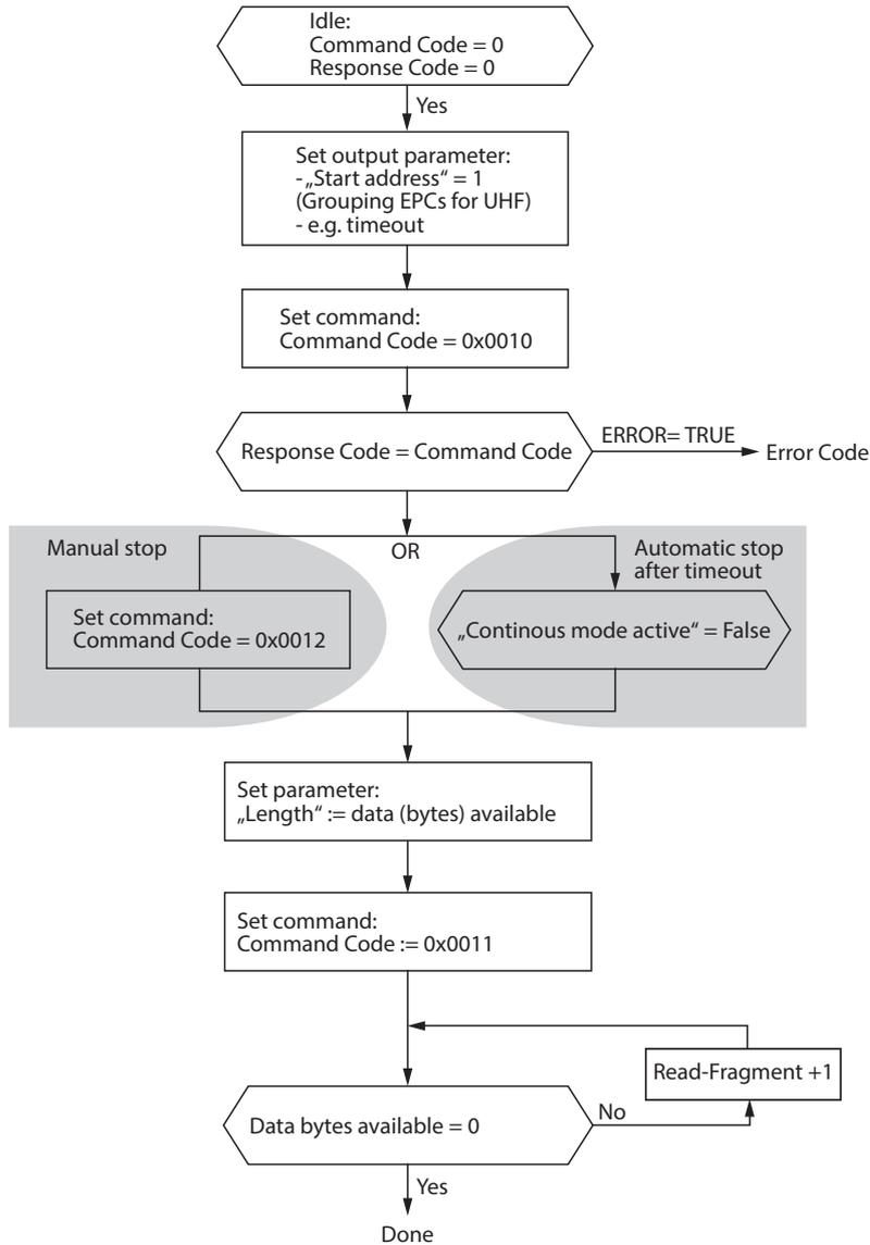
Fig. 58: Flow chart for Continuous Mode with interruption before reading data
