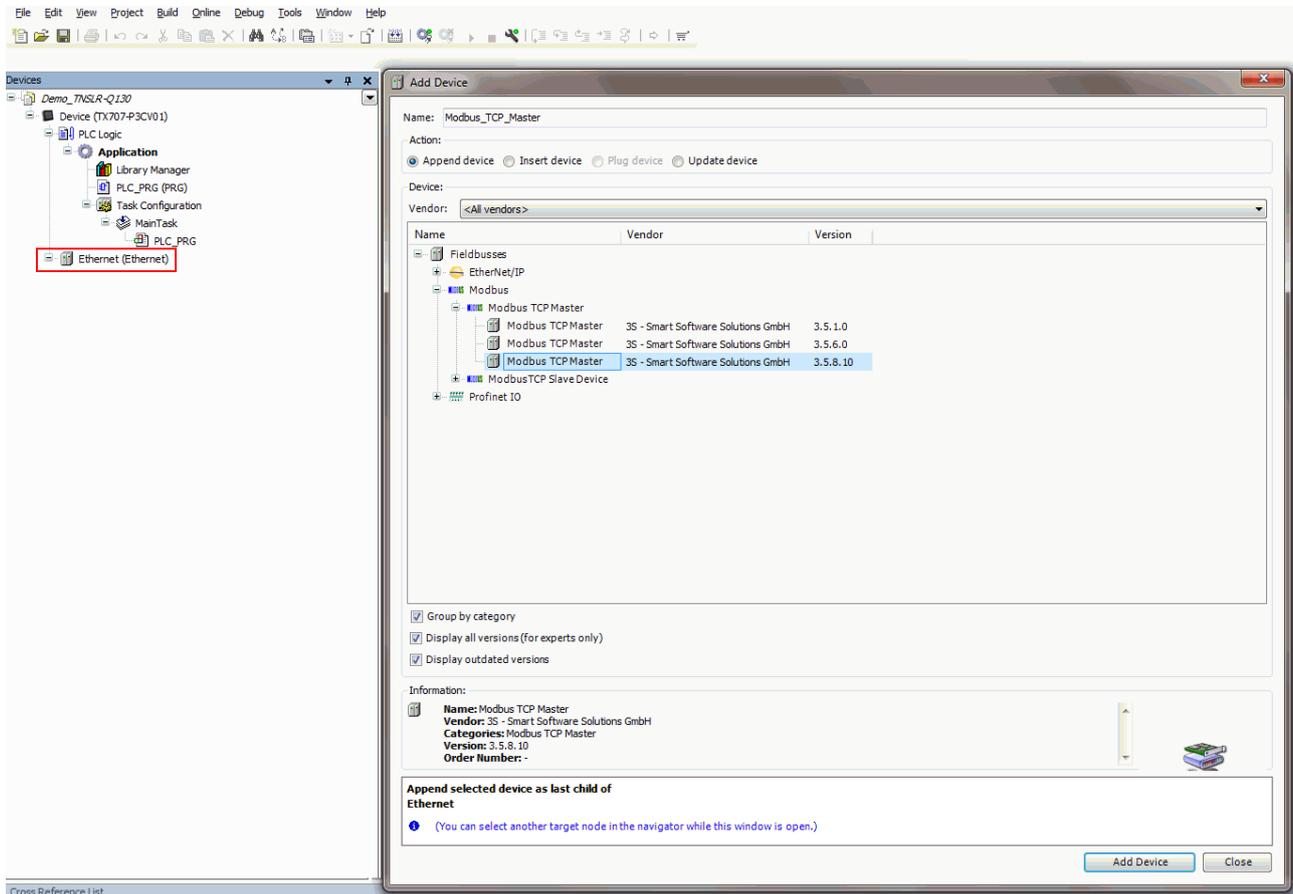
Fig. 16: Adding a Modbus master
