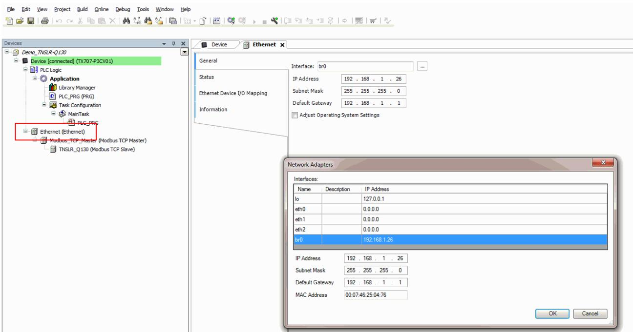
Fig. 20: Modbus master – Entering the IP address (here: 192.168.1.25)
