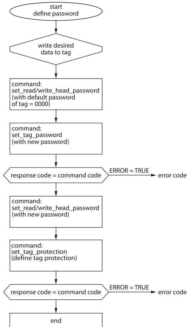
Fig. 60: programming tags with a password
