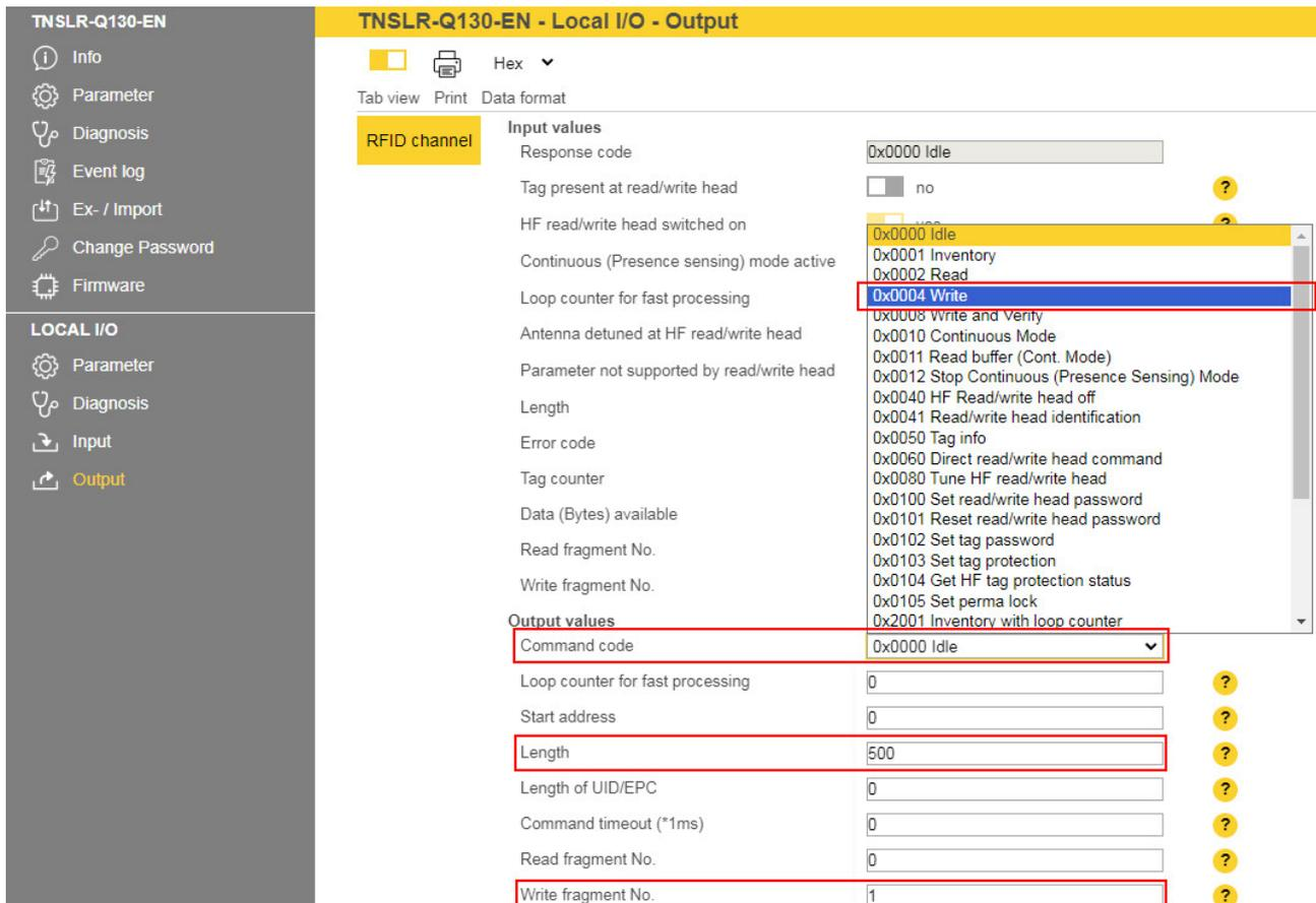
Fig. 49: Fragmentation – executing a write command
