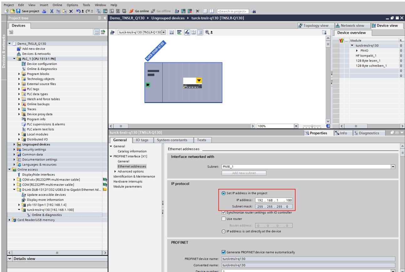
Fig. 37: Assigning the IP address
