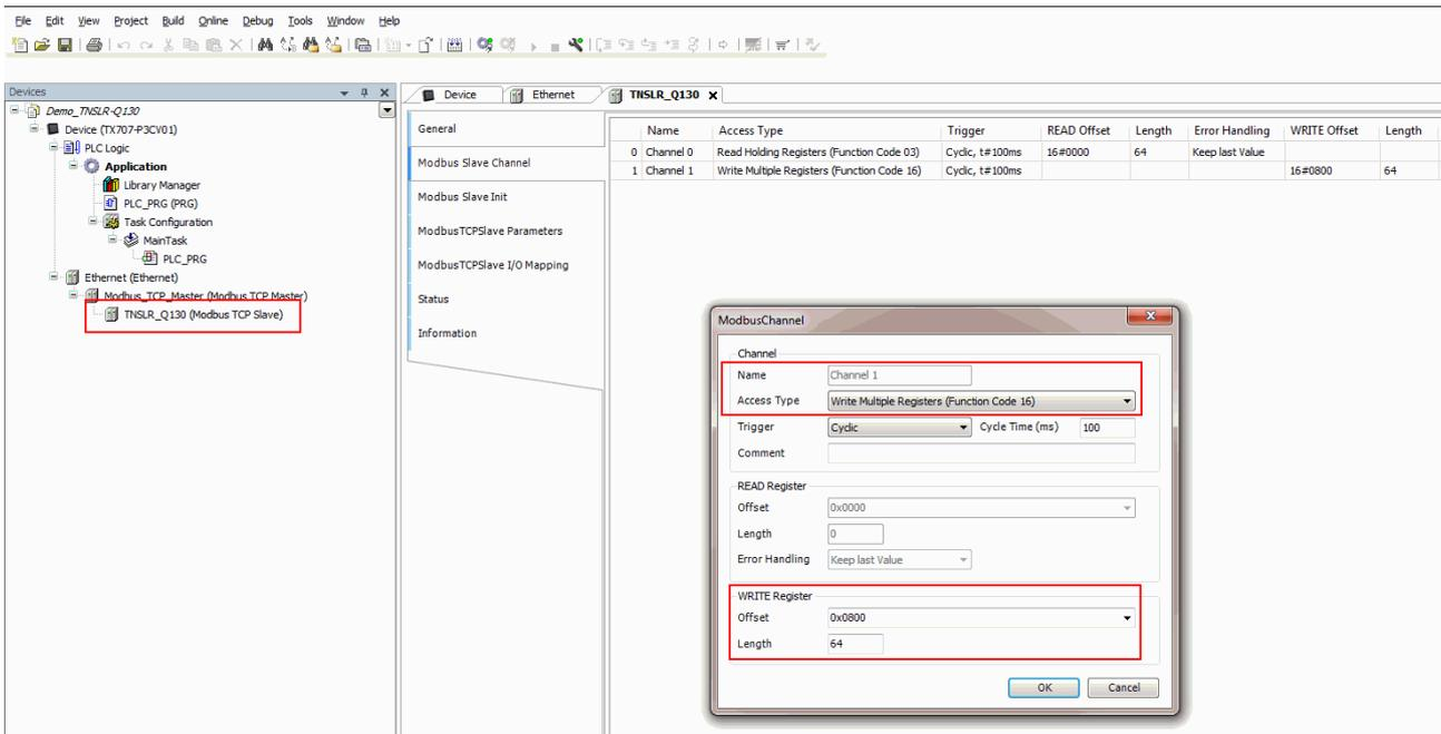
Fig. 23: Setting the WRITE registers
